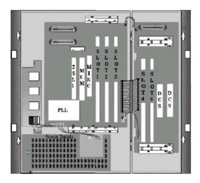
Figure 2–2 KSU With Expansion Type "B" Cabinet
